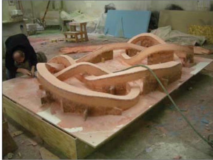
Giant Knot fabrication - fiberglass coating and phosphorescent paint application.
