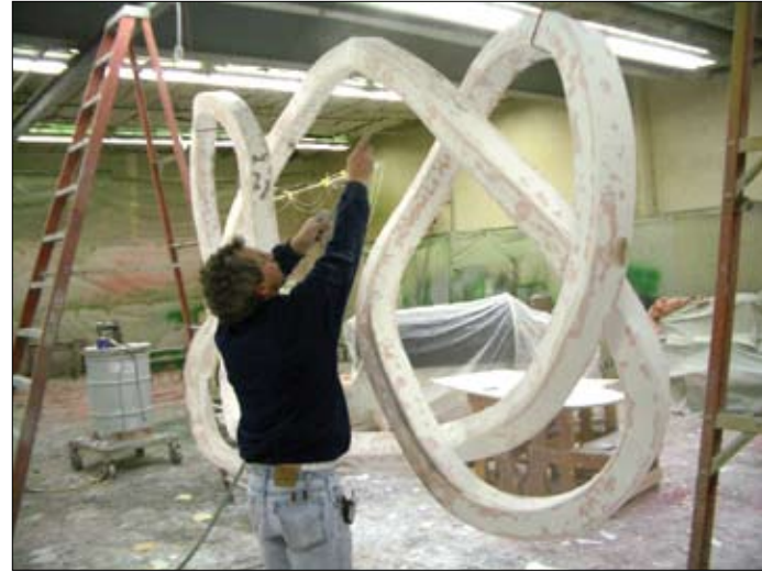
Giant Knot fabrication - fiberglass coating and phosphorescent paint application.
